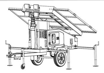
1. Please turn off the breakers for solar panels and batteries. Then disconnect the solar panels with connectors (B) on the trailer enclosure.
