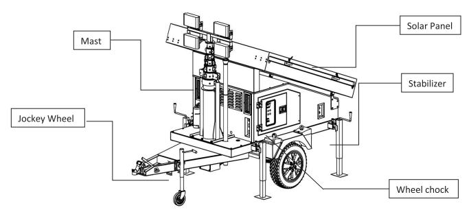
1. For maximum light coverage, locate the unit at ground level or in a spot higher than the area being illuminated by the lamps.
