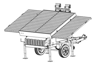
1. Unlock the solar panels (A) open the lock for solar panel (B) and pull the panels to the outermost position and make sure it is locked in place, and lock it
