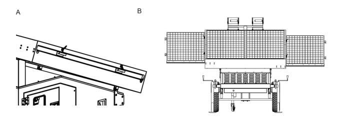
2. Connect the solar panel connectors to those plugs on the cabinet. Turn on the breakers for solar panels and batteries on the control panel.
